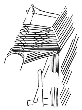
**Figure 2.** Detail of weaving on the warp-weighted loom in progress: Heddles attached to the heddle-rod pull warp-threads forward towards the weaver to create the artificial shed opening. Drawing by Gerassimos Bissas.
