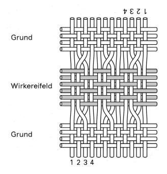
Fig. 10. Diagram of a typical example of the structure of *croisage*. After Schrenk (2004), 489, with permission.
