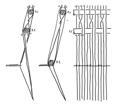
**Fig. 9.** Drawing showing the grouping of warp yarns on the loom for *croisage* (warp crossing). Drawing by courtesy of D. De Jonghe.
