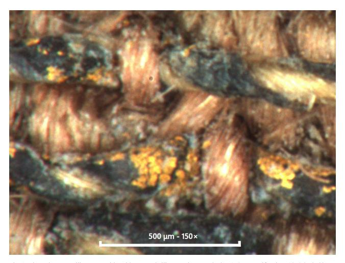
Fig. 1. Figured pattern silk woven with gold-wrapped silk yarn photographed at 150× magnification, 1950.2 © Cleveland Museum of Art. Note that much of the gold finish applied to the strips has flaked off of the surface of the yarn. Photo by J. Galliker.
