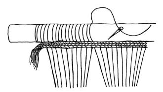
**Figure 3.** Above, detail of the starting border for a weave on the warp-weighted loom, showing the border sewn onto the cloth beam. Drawing by Annika Jepson. Copyright CTR.
