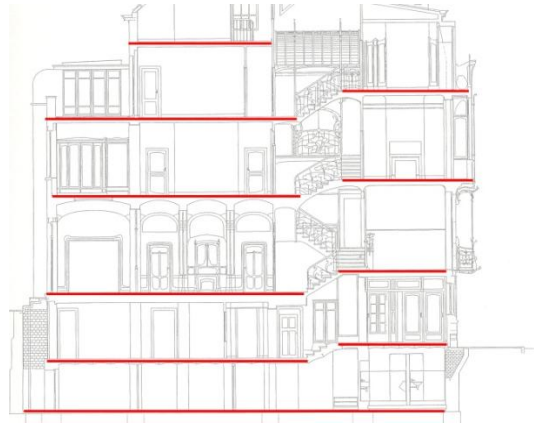
figure 6 : The personal residence of Horta is not constituted by floors, as by half-planes or parts of semi-levels and thus intensifying the phenomenal transparency.
