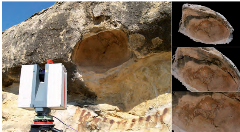
Fig. 3. Register by means of phase-shift laser scanning technology and photogrammetry of the Levantine rock art site called "Plano del Pulido" (Caspe, Zaragoza). On the right side there are different user-level software viewers from the model 3D.
