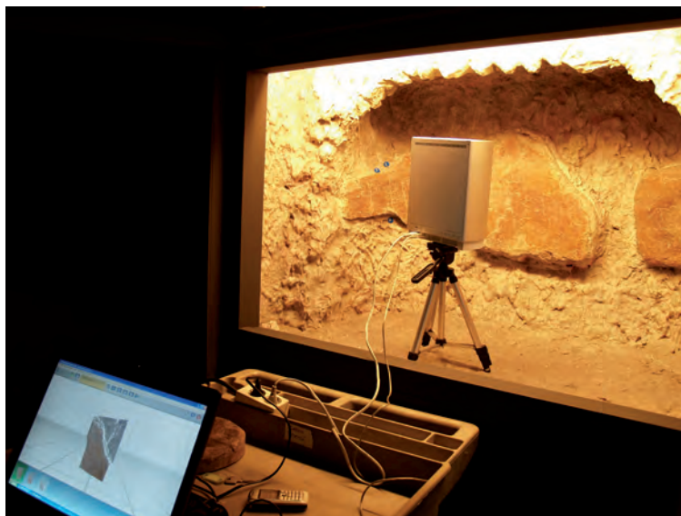
Fig. 4. Process of geometric data recording by means of triangulation-based laser scanning system. These rock art fragments were extracted from its natural site. Currently they are in the Archaeological Museum of Catalonia.
