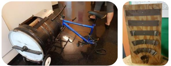
PICTURE 33: A MECHANICAL WASHING MACHINE AND A CORN SHELLER PRESENTED AT D-LAB SOURCE: AUTHOR'S OWN PICTURES
