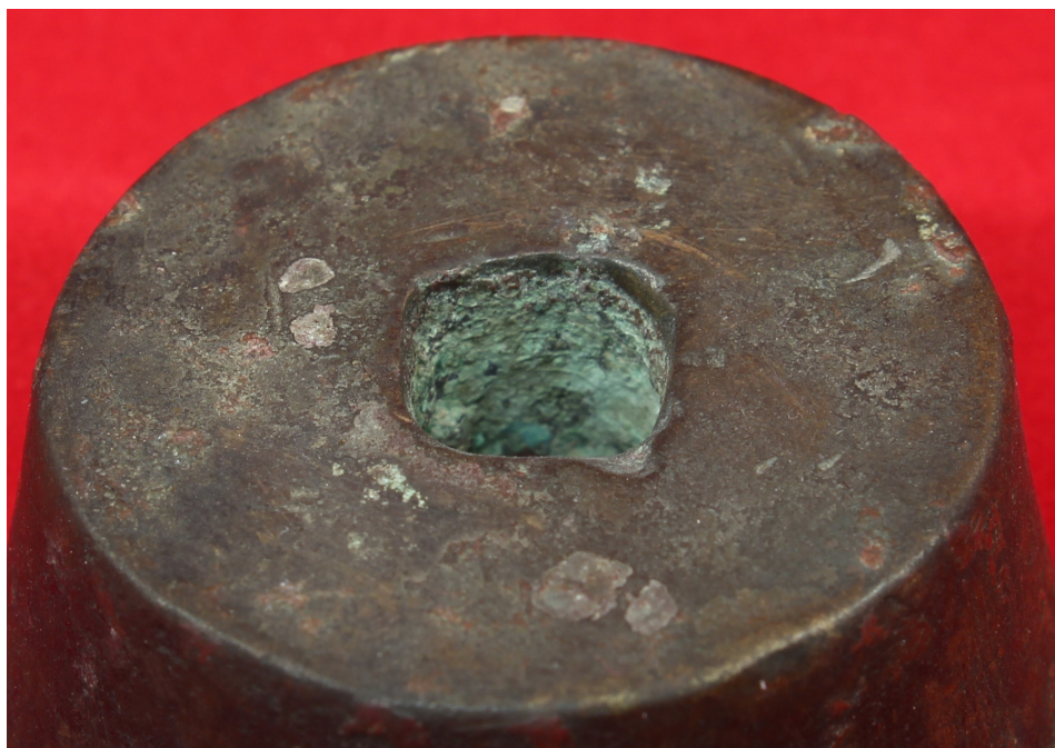
Figure 4. Detail of wear on one of the weights.
