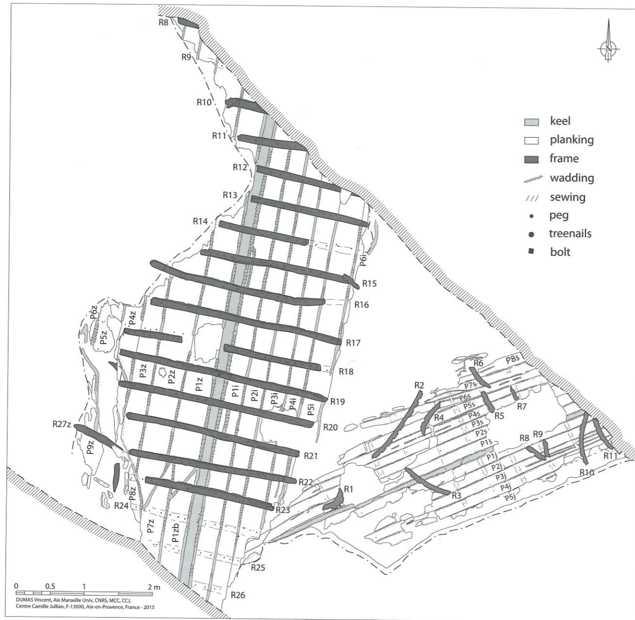
Figure 7: Plan of the two Roman shipwrecks of Pula (drawing: V. Dumas, G. Boetto, AMU/CNRS/CCJ).
