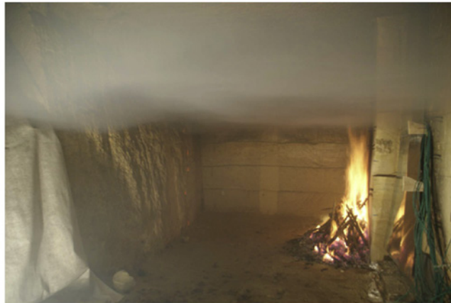
Fig. 11. Top: smoke distribution in the quarry during the fire (FDS) – bottom: smoke distribution during the experimental fire (credit: C. Ferrier).
