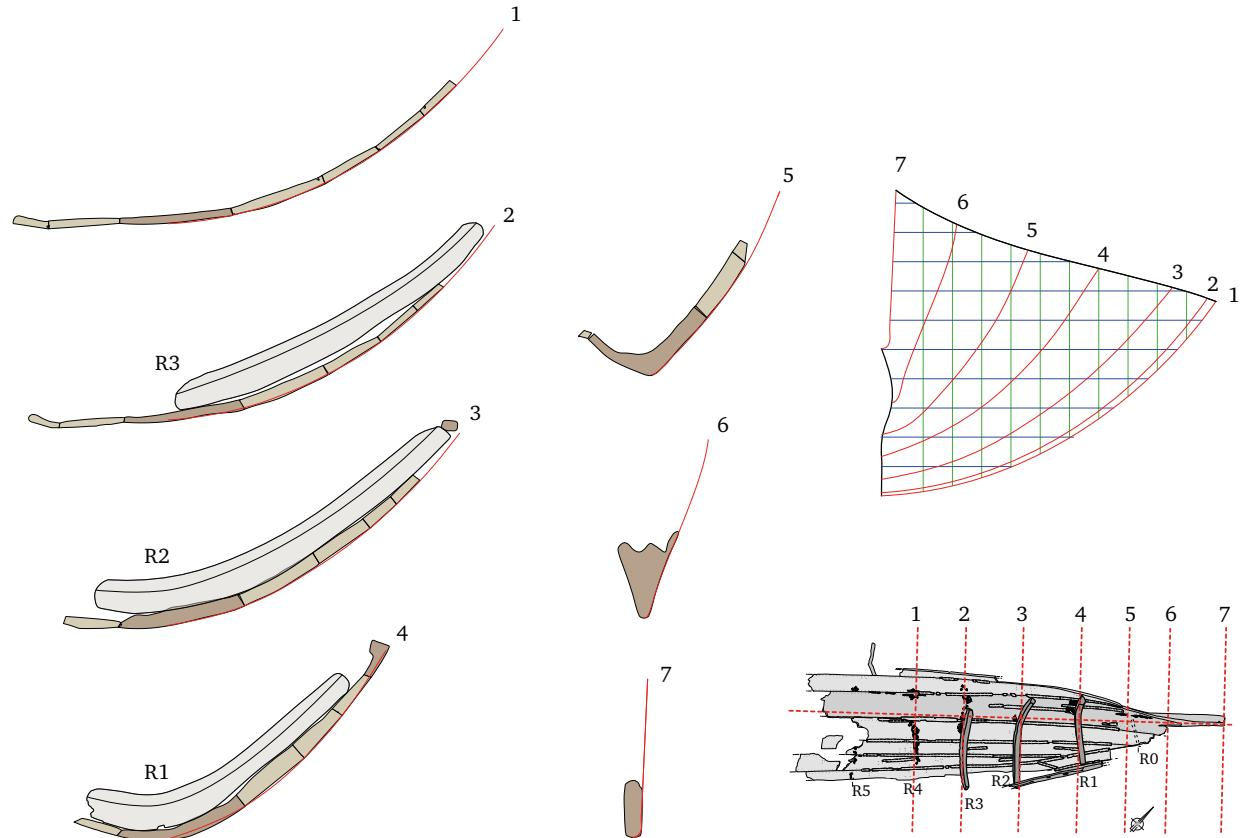
sel has a very pronounced bend or rocker along its length, matched by the curve of the sheer line, making it appear rather 'banana-shaped'.
