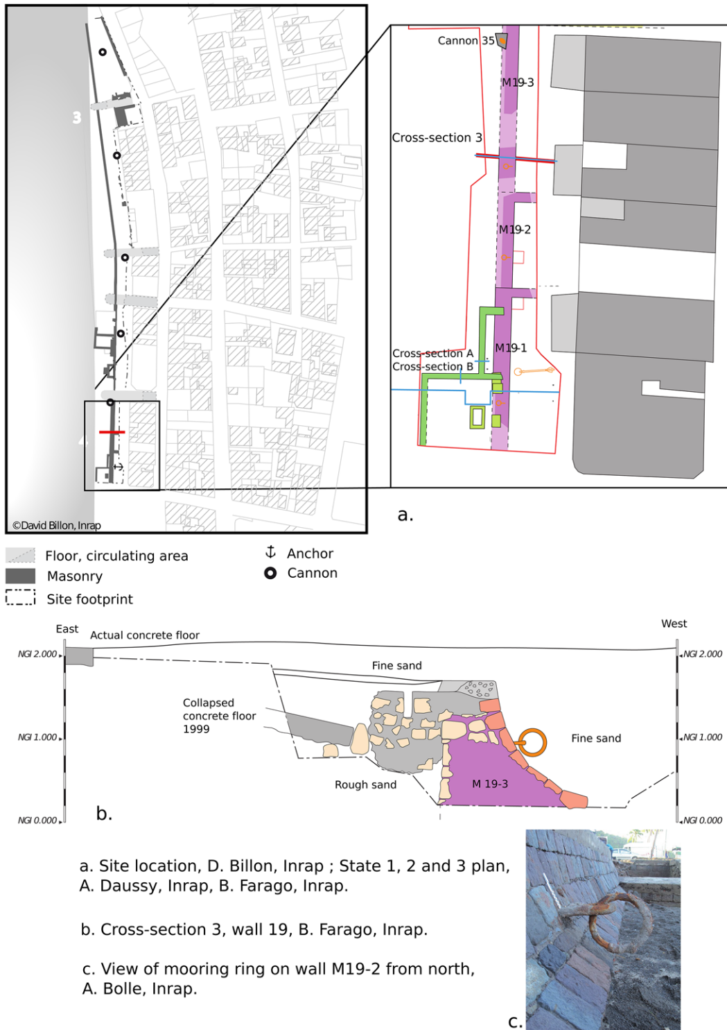
Figure 4. Seawall structure in Saint-Pierre (Martinique) (A. Bolle).
