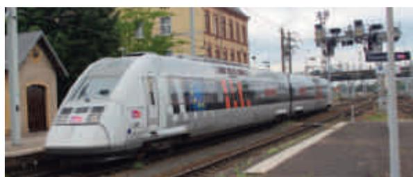
*X 72633/72634: the ETCS measurement and validation railcar*
