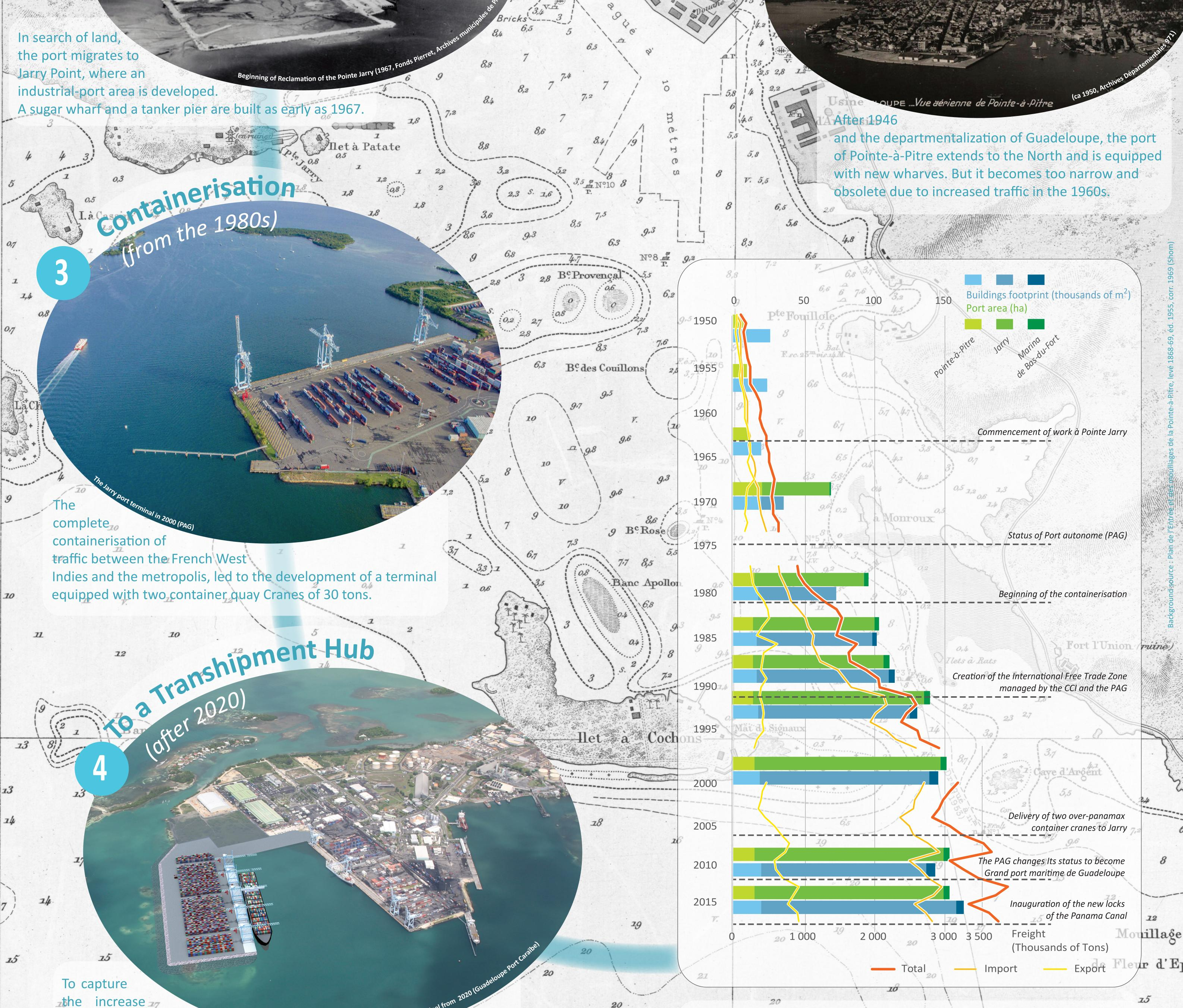
To capture the increase 17 in traffic expected after the expansion of the Panama Canal, the Jarry, terminal needs to be expanded. The project 22 involves a storage platform of 25 ha, 350 m of deep water docks, to accommodate vessels with a draft of 15 m.
