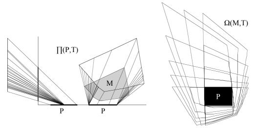
Figure 4: *M* is a section of  $\prod(P,T)$  (left and middle). The intersection of the shadows of *M* for all instants of *T* is equal to *P* (right).
