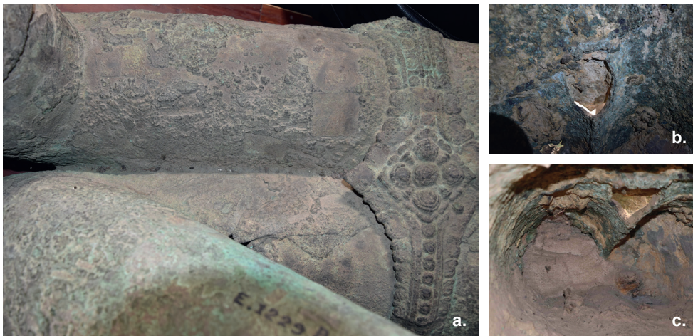
Fig. 11 — Wax-to-wax joins between the two right arms ( ga 5387): (a) view from above; (b–c) views from inside.
