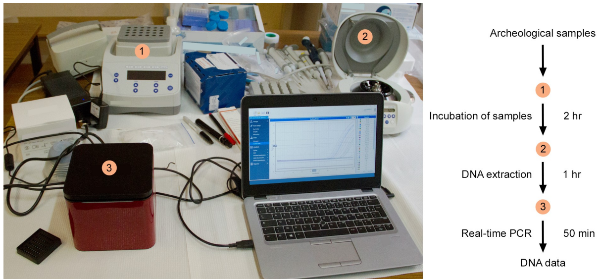
Fig 2. Overview of the device and experimental workflow. The left panel shows the heater-mixer used for sample incubation (1), the mini-centrifuge used for DNA extraction (2), and the real-time PCR instrument (3). The right panel summarizes the overall experimental procedure.
