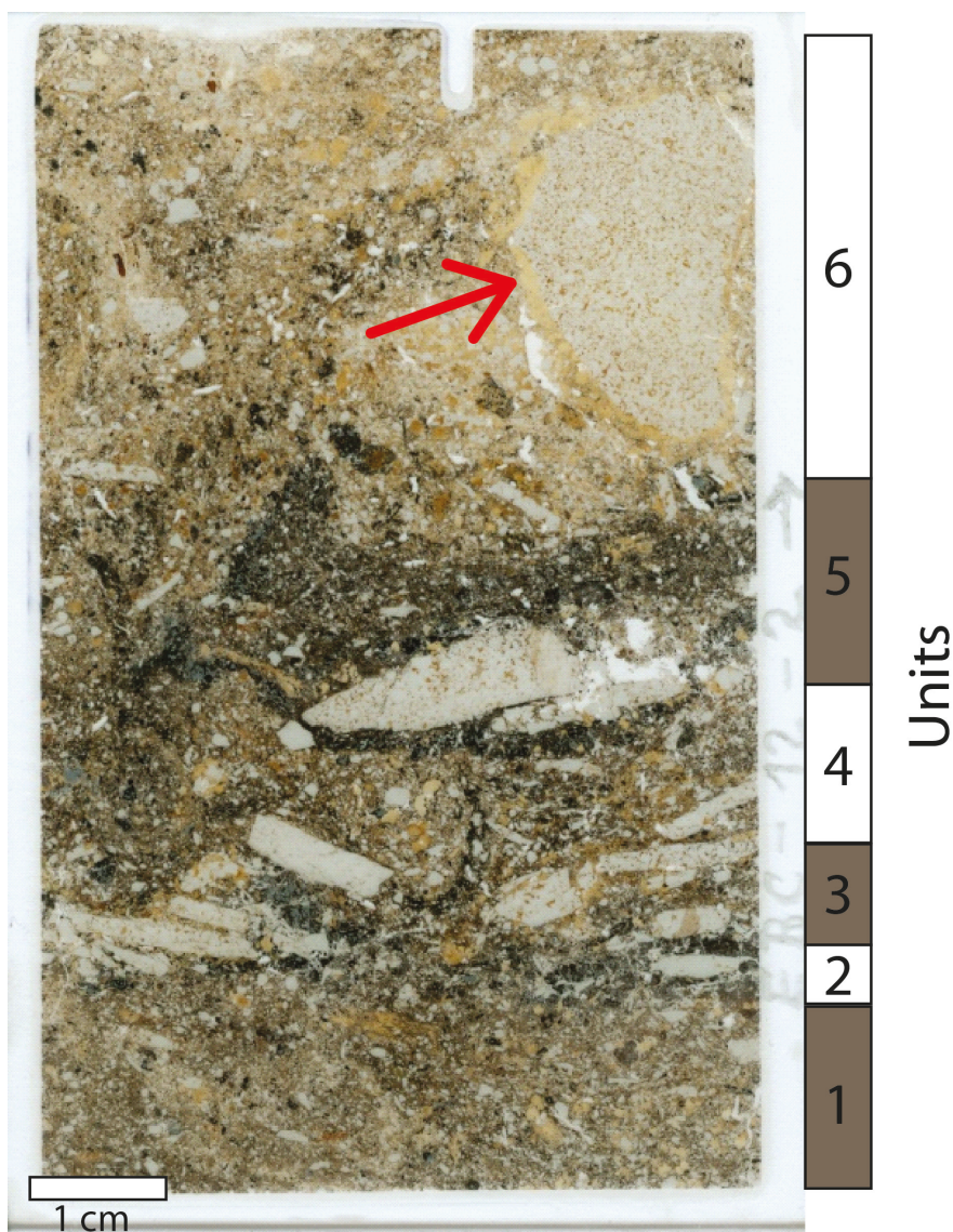
Fig. 11. flatbed scan of EBC-12-02 indicating the depositional units identified in thin section. Note the large block of quartzite around which a crust of taranakite has formed. Here one can see that units 2 and 5 are rich in charcoal, and unit 5 has a sharp lower contact.
