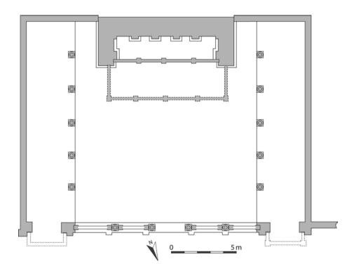
Fig. 7: Sbeitla, Northern Fountain, plan of the original construction presenting the hypothetical draw basin. Two porticoes frame the courtyard.
