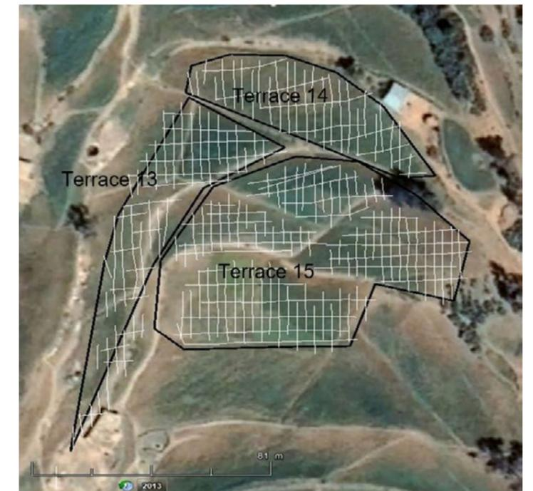
Figure 26: Profiles and tie-lines on terraces 13, 14, and 15 (R. Al Khatib Alkontar, H. Reiller – MAFTOr/IPGS-EOST).
