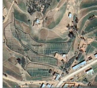
**Figure 11:** Profiles and tie-lines on terraces 1, 3, and 4 (R. Al Khatib Alkontar, H. Reiller – MAFTOr/IPGS-EOST).
