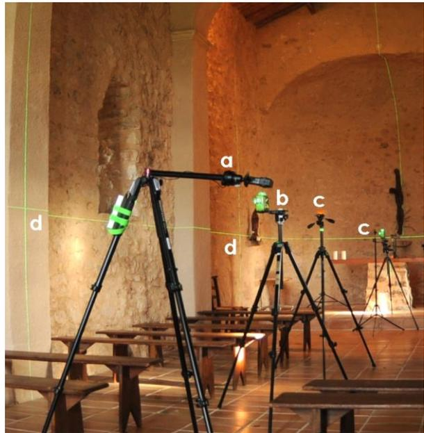
*Fig. 3. A sample setup: a the 360 camera; oriented horizontally, b a laser level, c tripods on which acoustic devices will be mounted, d intersection of laser beams on the envelope.*
