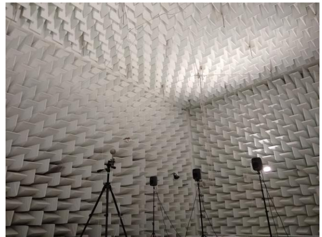
Fig. 4. The 32-way eigenmike and speakers positioned for reference tests in an anechoic room.).
