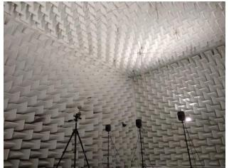
*Fig. 4. The 32-way eigenmeike and speakers positioned for reference tests in an anechoic room.).*
