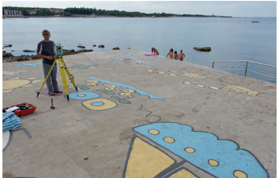
I.61 Georeferenciranje olupine Zambratija totalnom stanicom prema fiksnim točkama na obali Georeferencing the Zambratija wreck from fixed points on land using a total station (fotografija / photo by: Ph. Groscaux)
