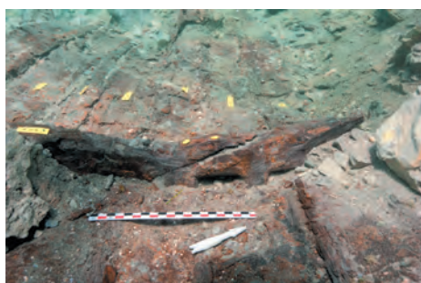
Fig. 40: Southern part of frame F10 from the East. The futtock (at the left) is overlapping the floor-timber and two vertical treenails (yellow pins) join the two elements (photo L. Roux, AMU, CNRS, CCJ).
