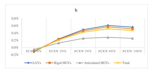
**Fig. 3.** Variation from the reference scenario of : travel time (a) in hour and distance traveled (b) in Vehicle kilometers (VKMs); Source: authors' calculation from VISUM
