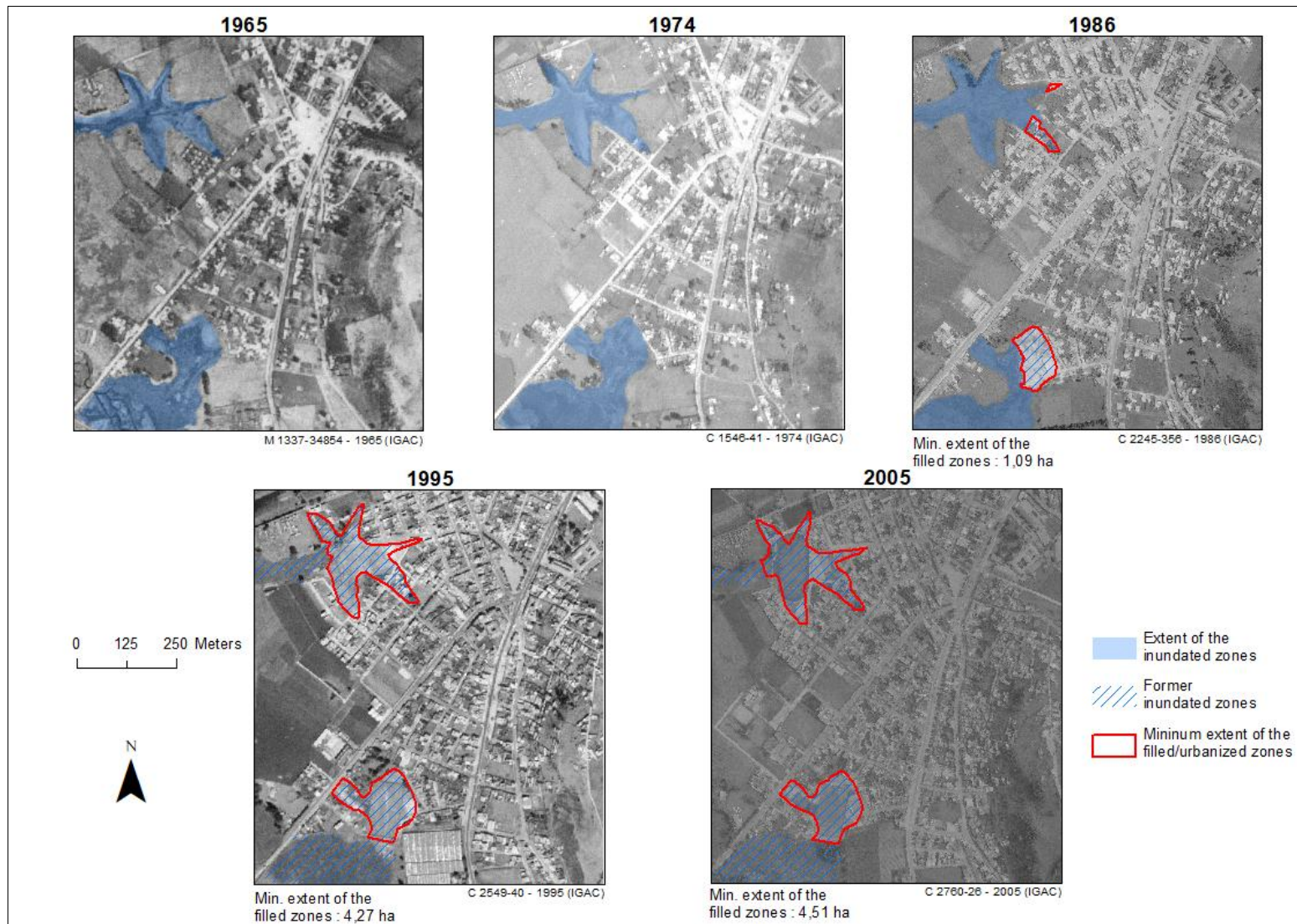
Fig. 4: Analysis of the desiccation of the reservoir's southern and western water intrusions in the urban area of Sibaté using aerial photographs
