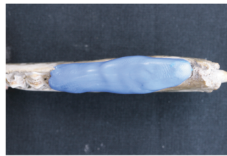
Second layer of putty silicone serving to support the mould
