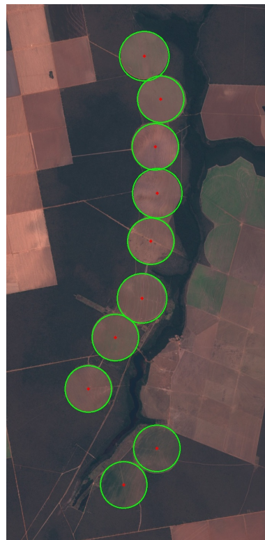
Figure 6. Center pivot irrigation systems accurately detected by Hough circle detection.
