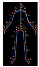
Fig. 4 Local features represented by the lengths of different parts of the skeleton.
