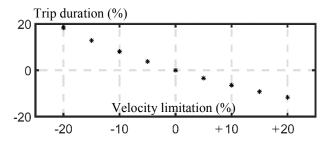
Fig. 14: Travelling time vs. velocity limitations
