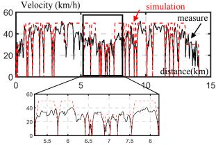
Fig. 9: Measured and generated velocities for the urban trip
