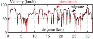
Fig. 10: Measured and generated velocities for the suburban trip
