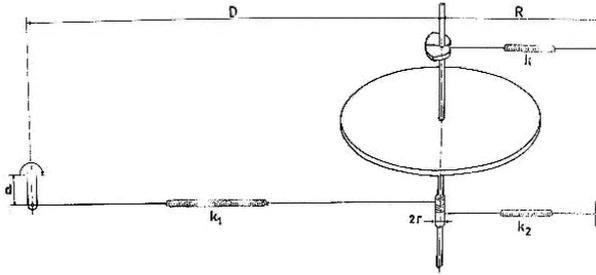
Figure 3: Outline of the geometrical aspects of the oscillator.
