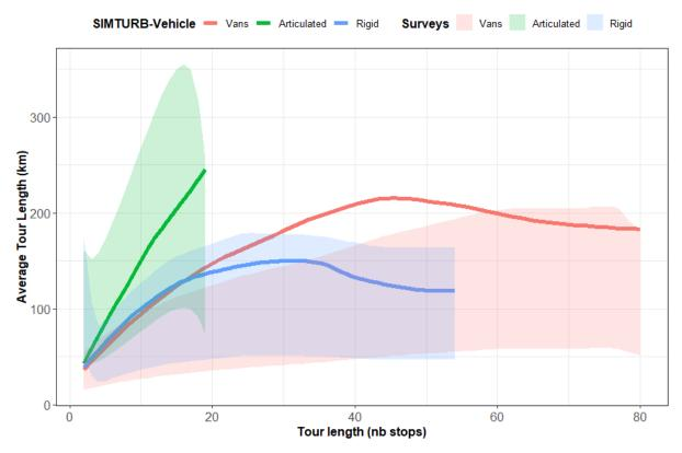
Figure 6 : total distance of a tour according to the number of points for types of vehicles, envelopes for survey values
