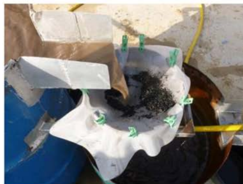
Figure : The light fraction is gathered with a sieve
