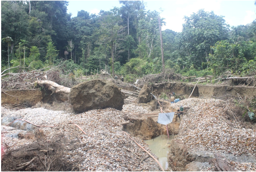
Fig. 4 A wildcat gold mining placer in French Guiana. The motor visible in the middle of the image pumps the sediments produced with the pressure jet and throws them into the sluice
