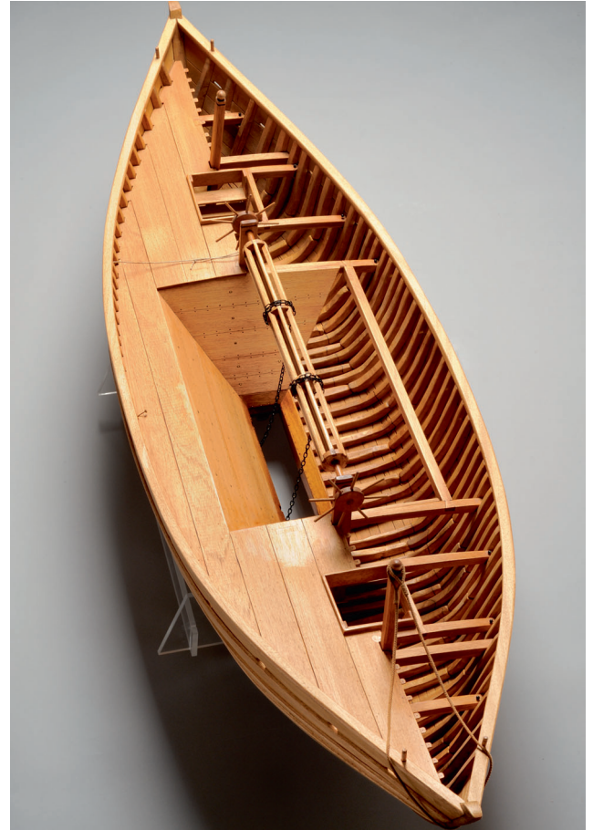
Fig. 5: Model of a Roman hopper barge (modelling R. Roman, photograph L. Damelet CNRS, CCJ).
