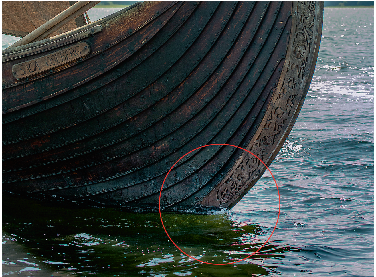
Fig. 4: When Saga Oseberg is in trim, stem ornamentations terminate above the water surface both fore and aft: does the ornamentation mark the ship's original trim? (photograph Werner Karrasch, the Viking Ship Museum in Roskilde, Denmark).
