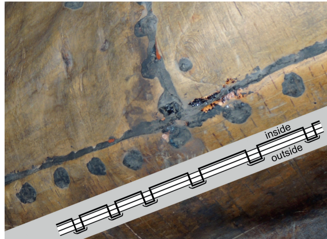
Fig. 5: Running stitch seam with short segments on the outer face of the canoe. Each short segment is made watertight by covering it with a large dot of black mastic (Yakut canoe, Siberia) (photography B. Arnold).
