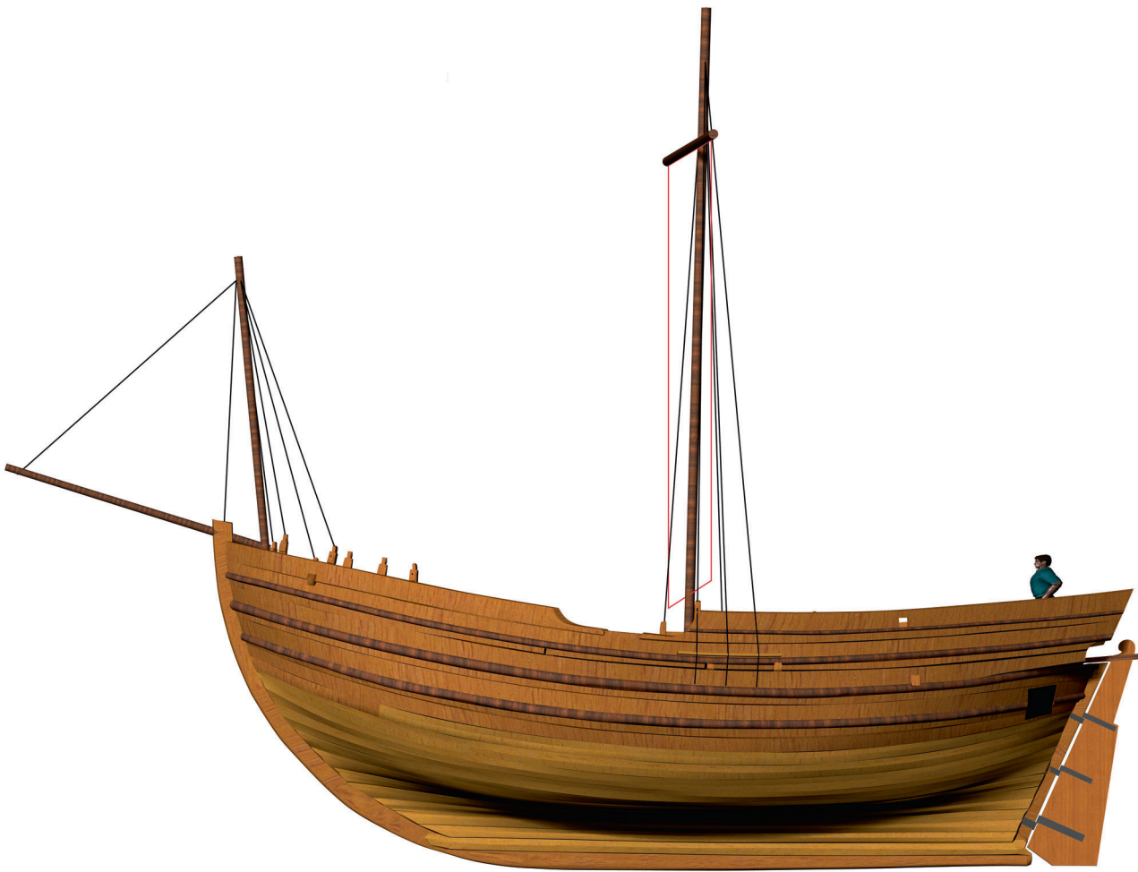
Fig. 1: Reconstruction of Barcode 02: bottom part of the hull in pine, upper part in oak. The ship is 14.5 m long.
