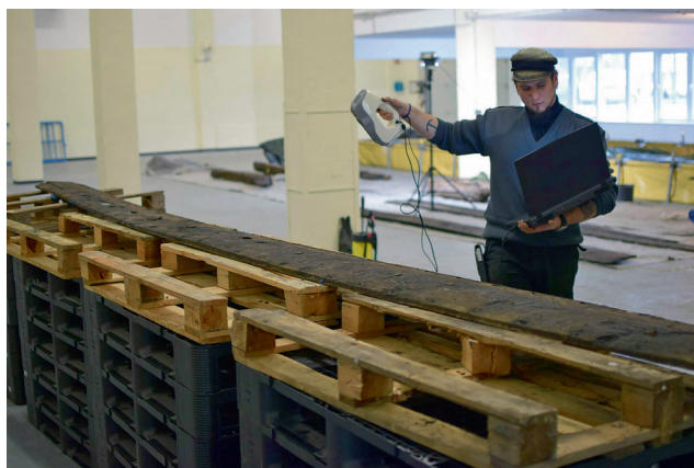
Fig. 1: Timber scanning setup using the Artec Eva structured-light 3D scanner (photograph T. Van Damme).
