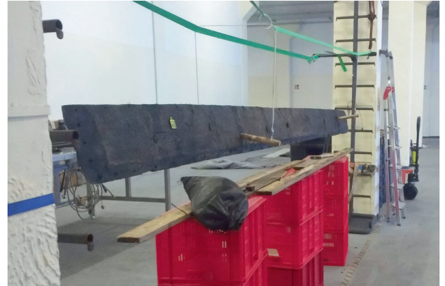
Fig. 2: Generally, planks will bend slightly when turned over, meaning that the 3D geometry of the plank changes in between two scans. This may lead to reconstruction errors when merging the outboard and inboard scans of a plank. In order to avoid this issue, planks can be suspended above the recording surface, thereby allowing the user to record the entire plank in a single scan (photograph J. Auer).
