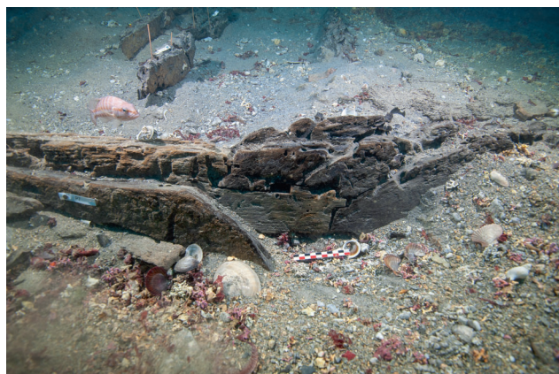
Fig. 4: The scarf between the keel (left) and the post (right): the garboard in the foreground (photograph L. Damelet, CNRS/CCJ).
