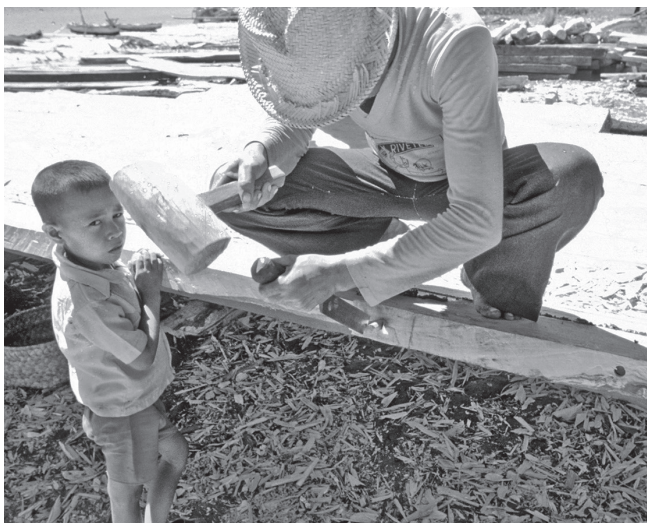
Fig. 4: Locking wedge in a pinisi from South Sulawesi (photo P.-Y. Manguin/EFEO 1979).
