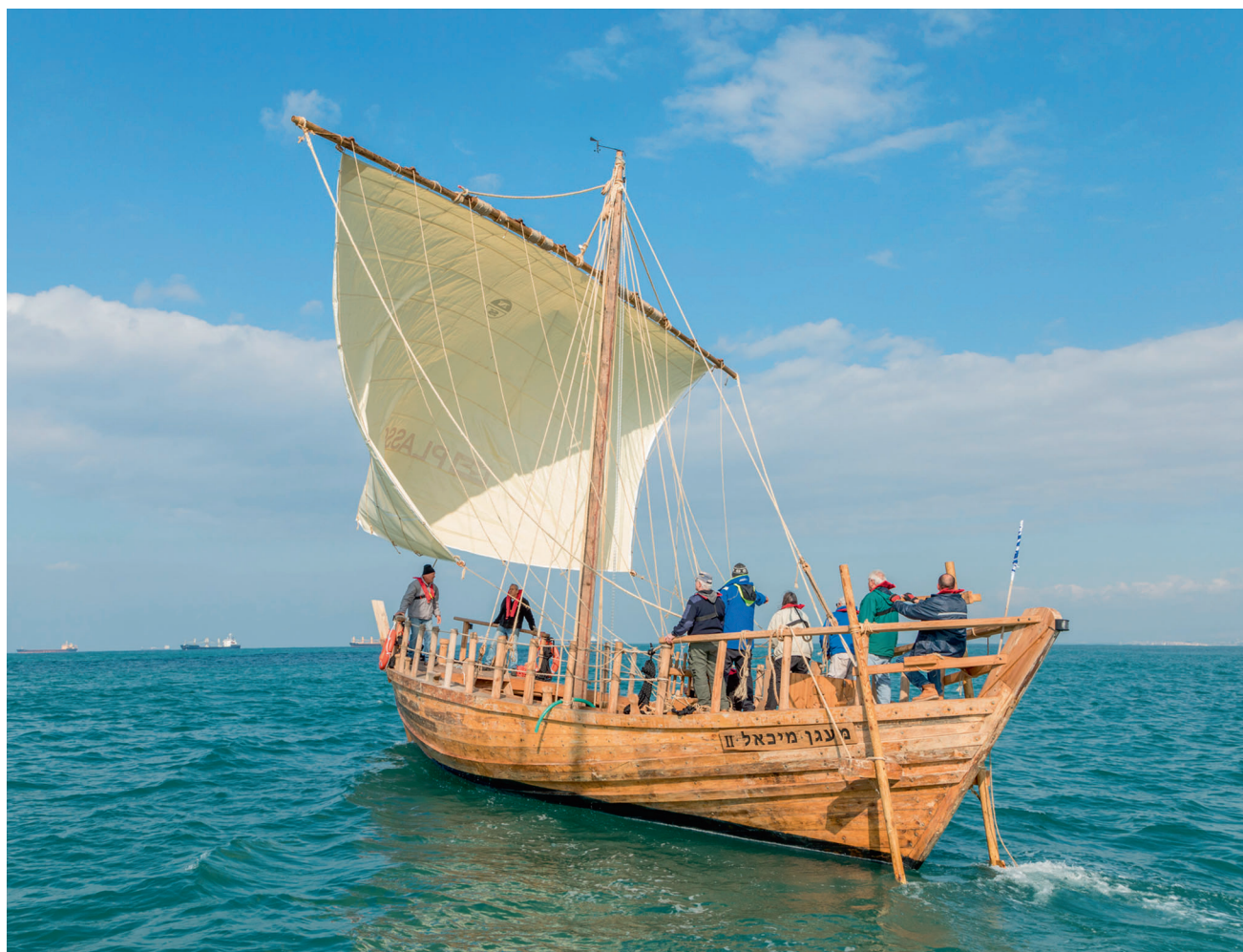
Fig. 3: The Ma'agan Mikhael II under sail on a broad reach. The two quarter rudders can be seen (photography E. Efremov).
