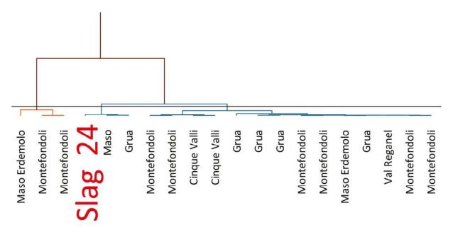
Fig. 5: Example of slag number 24: 97% similarity with the class and 99.5% similarity with the subclass.
