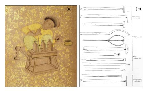
Fig. 2. (a) Lapidary using a bow-lathe to polish a gemstone. From an album of the Mughal emperor Jahāngīr, dated 1610–11 AD. (Prague, Náprstek Museum, MS A.12182, f. 16); and (b) tool kit from a traditional jade-carving workshop in Peking (Hansford [5], Figure 11, p. 81).
