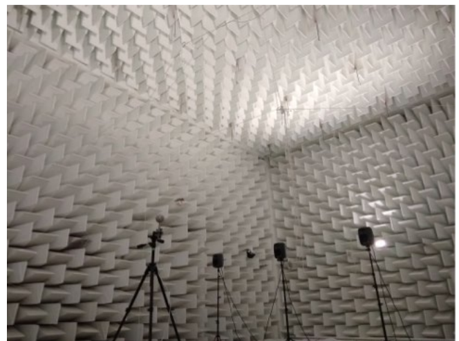
Figure 9. The Eigenmike 32 and speakers positioned for reference measurement in an anechoic room.
