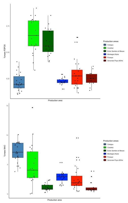
Fig 9. MnO and P<sub>2</sub>O<sub>5</sub> content of slag from the production areas.
