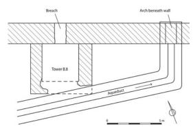
Fig. 6. Leptis Magna: passage of an aqueduct under the Byzantine walls next to tower B.8. (After Goodchild and Ward-Perkins 1953, 63.)
