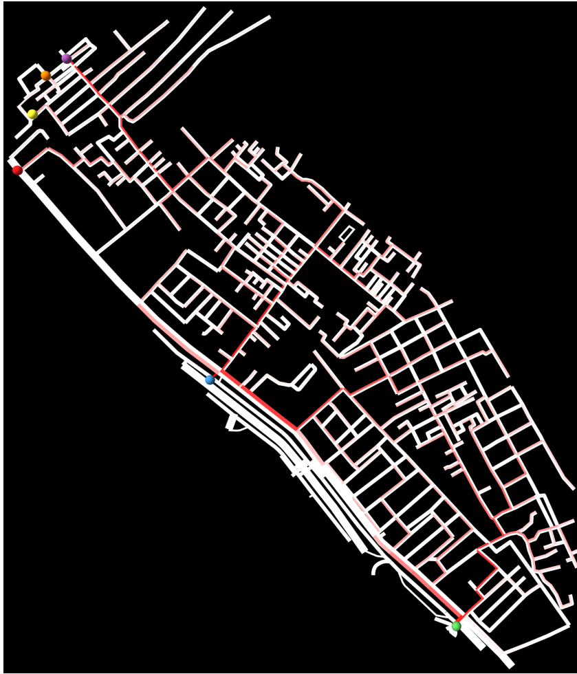
Figure 11. Road network displaying the shortest path between a building, and its closest evacuation point. The width of the road is proportional to its number of lanes. The spheres represent the evacuation points. The color of roads depends on the number of times they have been part of a shortest path to an exit point: the more it is red, the more it is supposed to be used by the agents to clear out the area.
