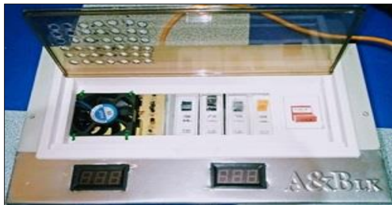
Figure 3: Constructed Hybrid Distribution Board Unpowered. Source: Authors, (2021).
