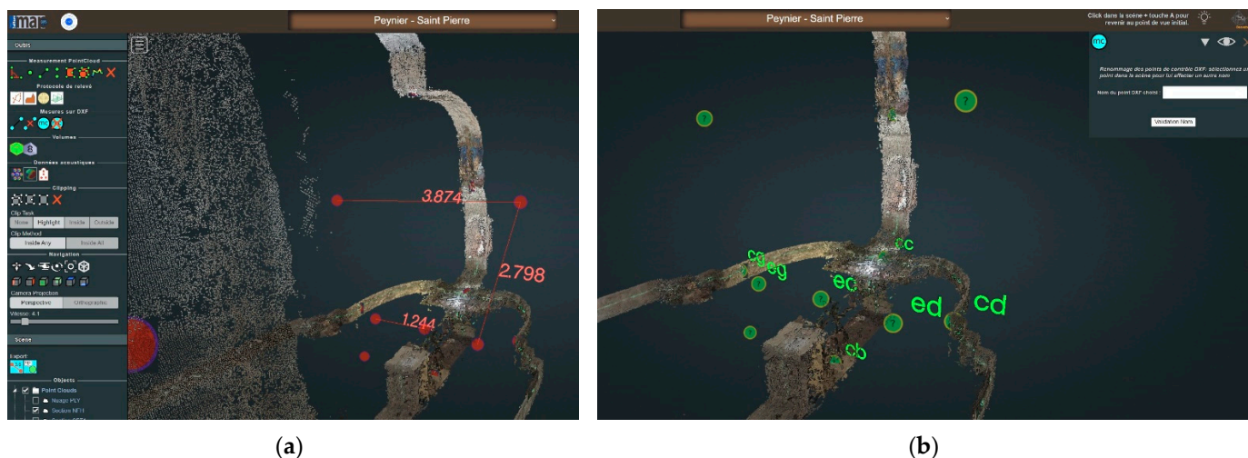
Figure 5. (a) Example of measurements made on the DXF data; (b) example of naming of DXF points in progress.
