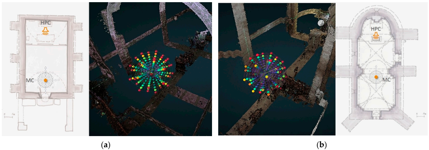
Figure 15. Clarity values for the MC/HPC tuple, showing all frequencies. Note in (a) high values (dark red) distributed all around the visual metaphor, in a first analysis attributed to the position of the microphone (very close to the entrance wall of the chapel, the smallest building in the collection (Saint Etienne Chapel, Sainte-Martin de Pallières, survey date 22 November 2019). By contrast, in (b), values on the rear side of the visual metaphor (yellow and green) show significant differences with those of the front side (dark red): the microphone, in this bigger building, is placed halfway between the entrance and the chancel (Saint Pierre Chapel, Peynier, survey date 11 December 2019).
