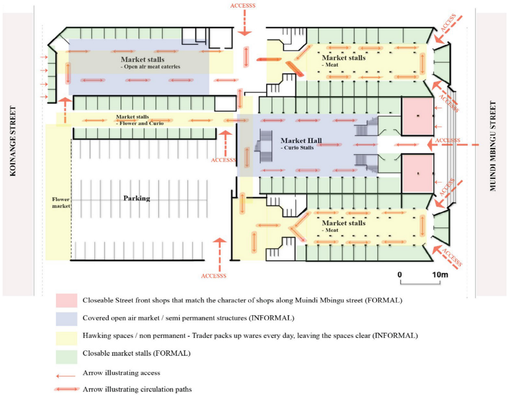
Figure 5.7. Spatial configuration and flow of movement in City Market. Drawn by author, 2020.
