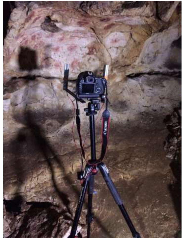
Instrumentation for UV photographs
