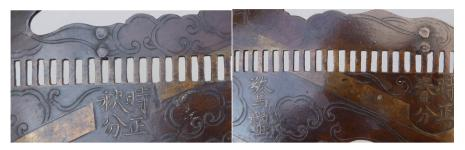
Figure 11. Equator, autumn equinox (left) and spring equinox (right); the equinoxes align with the two studs in each case.
