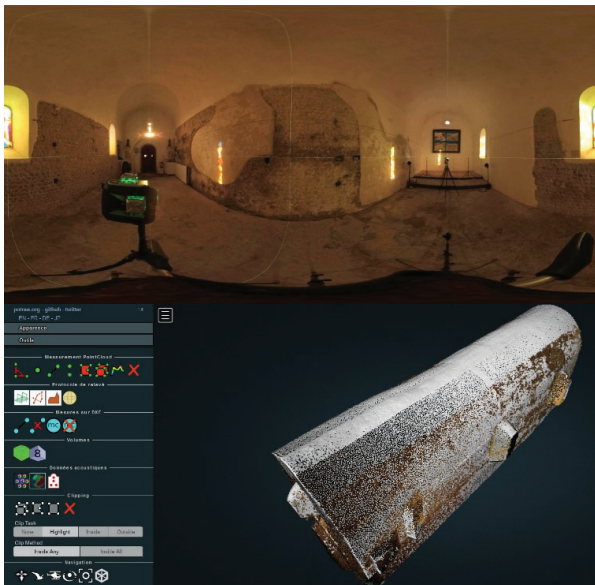
Figure 11. A case found to be critical for IBM (Saint-Roch chapel, Les Mées). Top, a stitch showing the predominance of white surface in the edifice. Bottom, the reconstruction, combining the photogrammetric model (brown points) and the laser scanner's output (white points).
