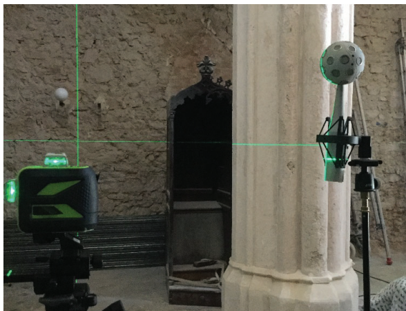
Figure 8. Vertical alignment of the Eigenmike 32 microphone, once positioned on the tripod in point MC, using the laser beams (N.D. de la Salette, Tourves).
