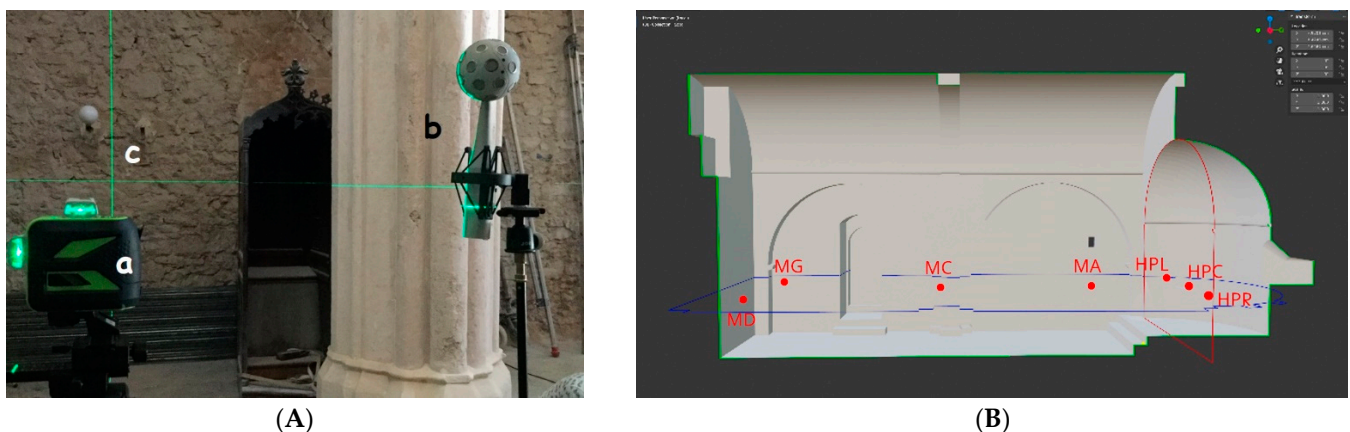
Figure 1. (A) The Eigenmike em32 microphone, (B), aligned vertically on the protocol’s spatial grid using laser beams emitted by self-levelling laser levels (a), and an intersection of laser beams used for the scaling step (c). (b) Illustration of the protocol’s spatial grid, with names given to emitting and recording points (Chapelle N.D de Bethléem, Bras, longitudinal section).
