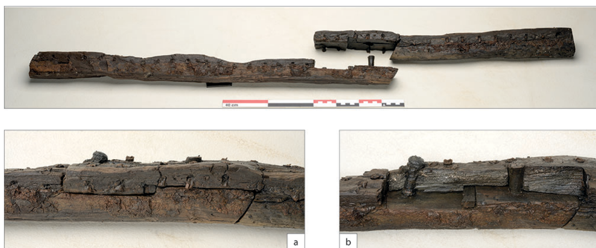
Figure 9. Poreč 1: The port side of the keel K (left) and transitional timber K2 (right), in the middle is the hook scarf; A and B) Details of the hook scarf with the horizontal key, the nail and treenail driven perpendicularly (photos, Ph. Soubias, CNRS, Aix Marseille University, CCJ).
